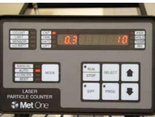
Met One laser particle counter is used daily to assess Hartley Medical's air quality.
